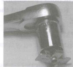
Figure 3 - Combustion Shutoff Device Assembly in 15/16" Socket on Wrench
