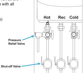
Instructions for pressure, temperature and vacuum relief valves shall specify that no valve is to be placed between the relief valve and the tank. The instructions shall specify installation in such a manner that the discharge from temperature and pressure relief valves will be conducted to a suitable place for disposal when relief occurs and that no reducing coupling or other restriction be installed in the discharge line.
