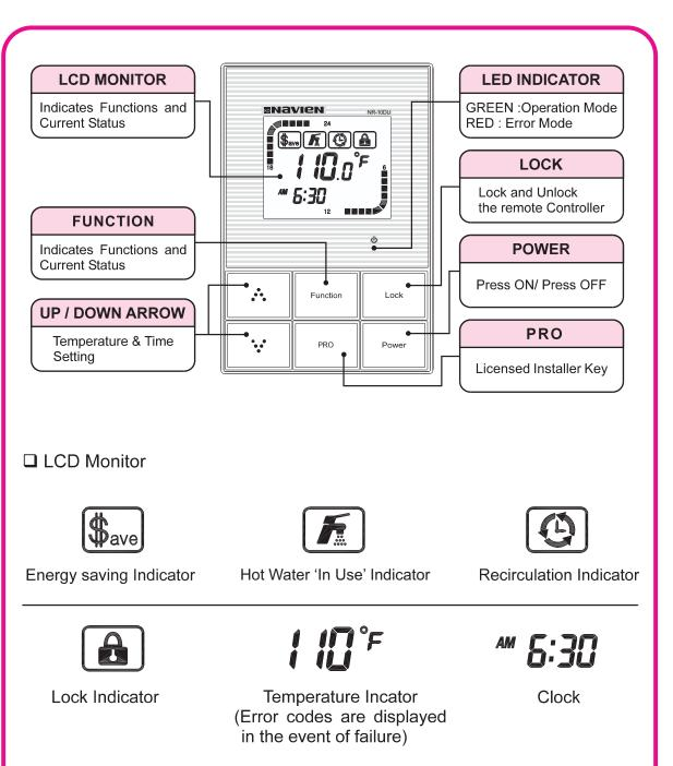
The Navien Remote Controller allows the customer to adjust hot water temperatures and to diagnose certain operating and fault conditions. The factory set temperature of the remote controller is at 120°F(NP Series: 140°F). Remove the protective sheet from the remote controller surface.
