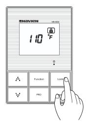
To engage and disengage the "LOCK" key feature, press and hold down the key for 3 seconds.
