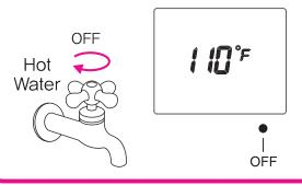
When the hot water faucet is closed, the water heater turns off automatically. The GREEN LED indicator turns off.
