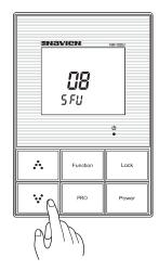
Press the "∴" or "√" button to adjust desired cascade OFF unit value. The value may be adjusted within the cascade ON unit setup value by 1.
