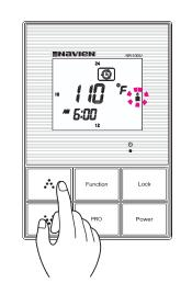
Press the : (Up) or : (Down) Key to adjust the cursor ' around the 24 hour clock in 30 minute increments. The 24 hour clock is displayed around the perimeter of the remote controller display screen.
