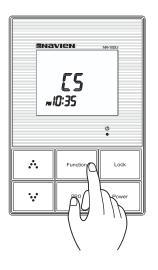
Once the "Function" button is pressed, "AM/PM" flashes on the display. Use the  $\therefore$ (Up) or  $\because$ (Down) buttons to select AM or PM. After 3 seconds, the selection is automatically set.
