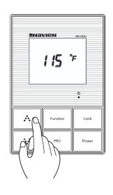
Press the  $\triangle :: (Up)$  or  $\triangle : (Down)$  button to scroll until the desired temperature is displayed on the LCD Monitor.
