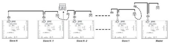
The Dip SW6(KDC-324-xM PCB Board), which is used only for organizing cascade system, Is to be switched Down if the corresponding unit is the first or the last unit of Cascade connection.
