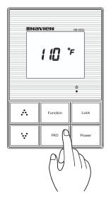
When the Pro Key is pressed for 5 seconds, high temperature adjustment mode is readied.
