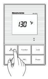
Each time ...(Up) Key is pressed for 3 seconds, temperature increases by 5°F. When the desired temperature is reached, leave alone and it will automatically set.
