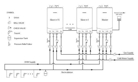
• In the status that recirculation piping connected to cascade piping are open, activate internal pump. If flow rate per a unit does not reach to 2 GPM, please check flow rate as closing ball v/vs at recirculation enterance one by one. At this time, please set the unit whose ball v/v is closed as internal circulation.
