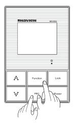
When you press the "Function" button and "Pro" button for 3 seconds, the setup mode will be over and it enter the power off mode.
