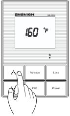
Each time Pro Key is pressed for 5 seconds in high temperature adjustment mode, temperature increases by 10°F (140~180°F) or 5°F (180~185°F). When the desired temperature is reached, leave alone and it will automatically set.
