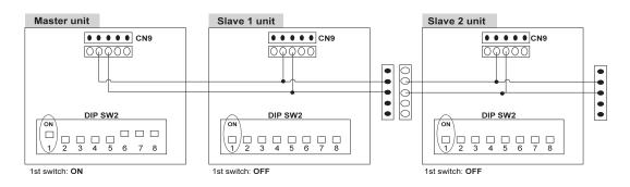
Cable connection and DIP switch set-up
