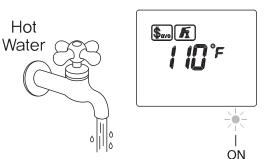
When a hot water faucet is opened, the unit will automatically start. The GREEN LED indicator will illuminate indicating normal operation.
