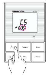
Use the  $\therefore$ (Up) or  $\because$ (Down) buttons to scroll until the desired minute time is reached. Press the "Function" button to set.
