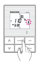
Reform Re When you press the function button at a desired recirculation start time, a ' $\blacksquare$ ' mark will appear meaning, that you are setting that time period for a circulation. After the black box mark appears, it will automatically go to the next time period, asking you if you want a circulation at that time, and so forth. You can manually press " $\cdot \cdot$ " or " $\cdot \cdot$ " to scroll to the time period that you want altered.
