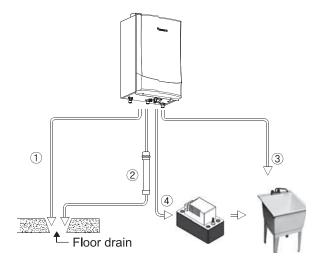
**Note:** Do not cap(or plug) the intergrated condensate line. Without proper drainage or disposal, condensate will damage the Navien Water Heater.
