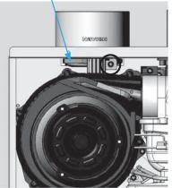
Remove the filter from the bottom of the intake air duct. Remove the Intake air filter from the plastic assembly and clean it with a toothbrush and water. Re-fit the screen into the plastic assembly and fit the filter and frame onto the bottom of the intake air duct.
